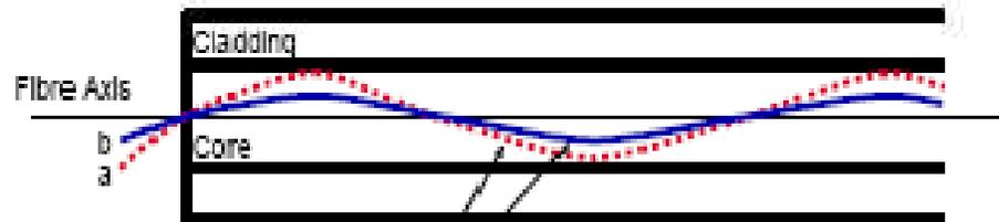
Light ray (a) and (b) are refracted progressively within the fibre. Notice that light ray (a) follows a longer path within the fibre than light ray (b)
