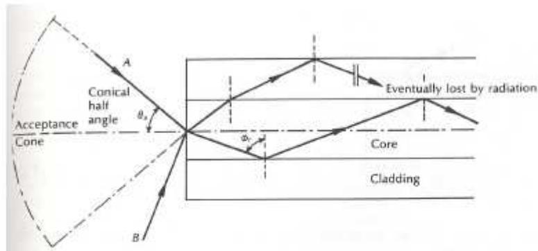
Coupling of a ray into a fiber. The ray can only be coupled into the fiber when the angle of incident is within the acceptance cone.
