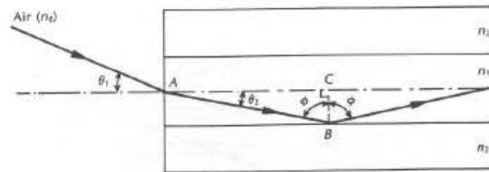
Coupling of a ray into a fiber. The ray can only be coupled in the fiber when the angle of incident is within the acceptance cone.
